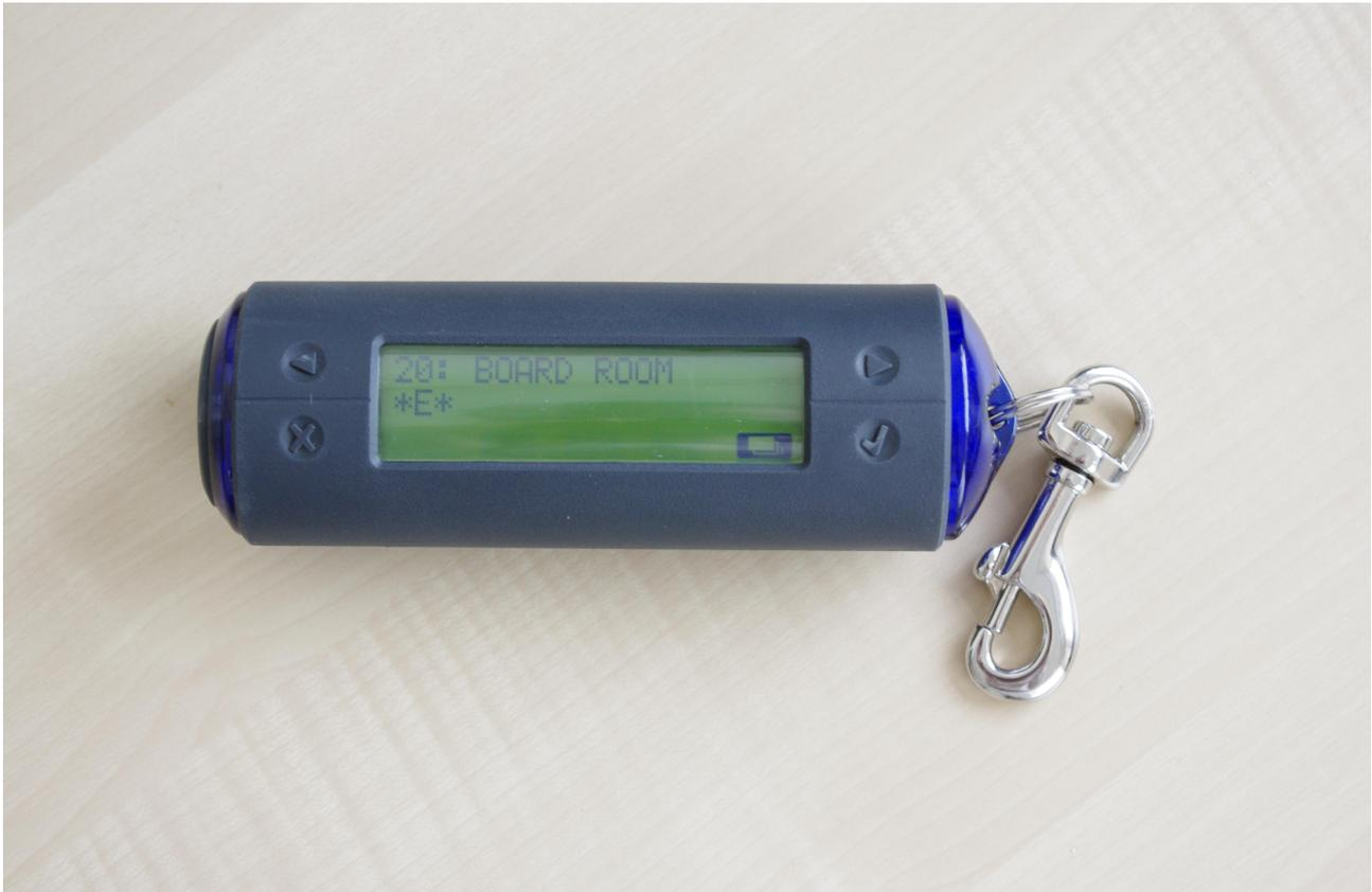
The Pinpoint PITpager is designed to operate with the Paging Transmitters installed with all Pinpoint and INSTANTalarm Staff Personal Alarm Systems. It provides the combined functions of a Personal Infrared Transmitter (PIT) and a portable Display Pager.
